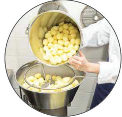
**Best for:** The bulk feed hopper enables continuous filling by the bucket load for preparation of primarily round products. Capacity is very high because the machine runs continuously and is therefore extremely time-efficient. The FP400i with a Feed Hopper can be beneficially included in a continuous production flow.
